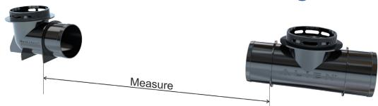
Slide a 5" clamp over the pipe. Apply a generous amount of silicone grease around the fitting and the inside of the pipe. Push the pipe on to the fitting. Use the supplied socket on an electric drill with clutch setting 5 to tighten the clamp. Ensure a gap is left between the flange and the clamp because if the clamp catches the flange it can crack the plastic.
