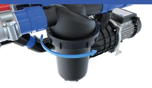
The water pump has a basket filter which catches larger debris. The secondary in-line filter has a fine mesh filter to remove smaller debris and organic matter. Both filters should be checked and cleaned when the system is empty, ideally when performing a nutrient change.
